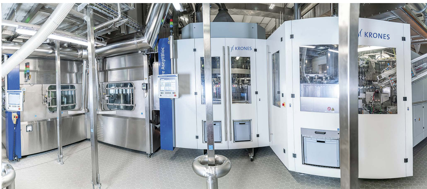
The heart of the new lines: the dry-aseptic blow-moulder/filler block (photo: Krones)
