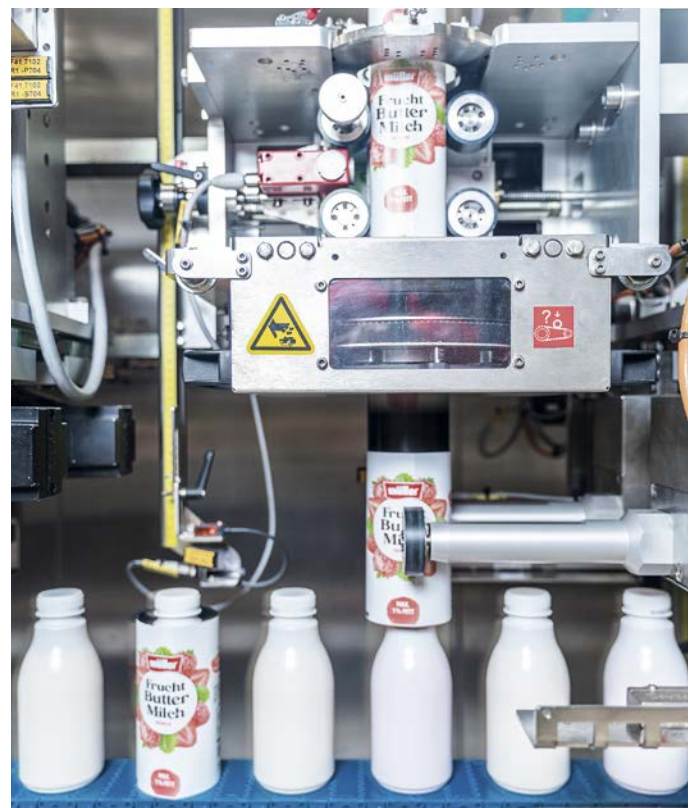
Two Sleeveomatic labellers dress the containers in sleeves (photo: Krones)
