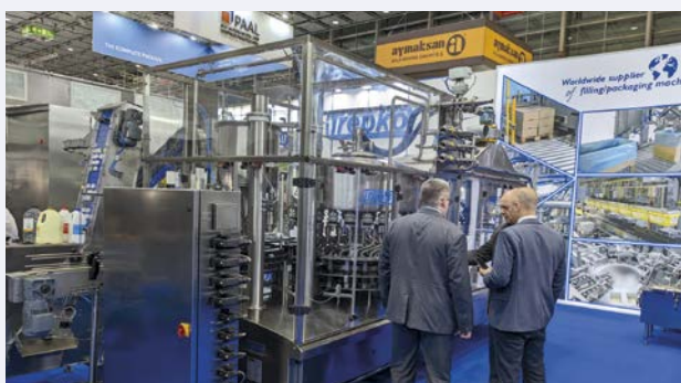
The new aseptic rotary fillers of the 200-A series from Trepko work with log 5.9 (photo: IDM)
