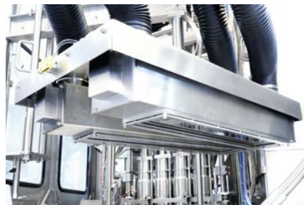
High-performance radiators of the double pulsed-light high-performance UV(C) sterilisation system in the hygiene tunnel of the ultraclean rotary-type cup filling machine
