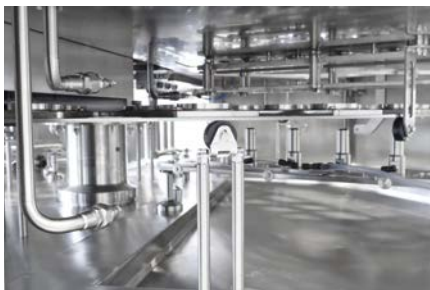
View of the interior; on the left one of the spraying nozzles of the fully-automatic interior cleaning for foaming and rinsing the rotary table; optional, supplementary equipment: complete interior drying with heated laminar air
