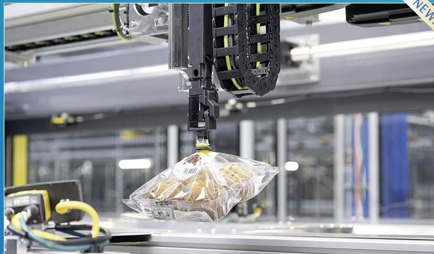
AI-based object detection plus state-of-the-art gripper technology ensure that goods are gripped securely and placed gently in target bins or cartons (photo: SSI Schäfer)
