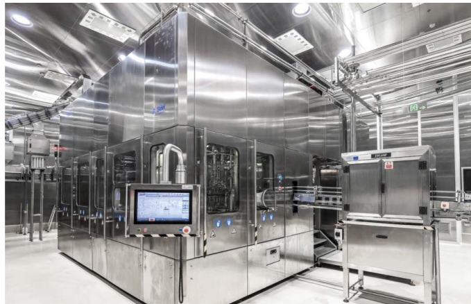
Yili has installed a versatile Aseptic Lab filler by Sidel (photo: Sidel)
