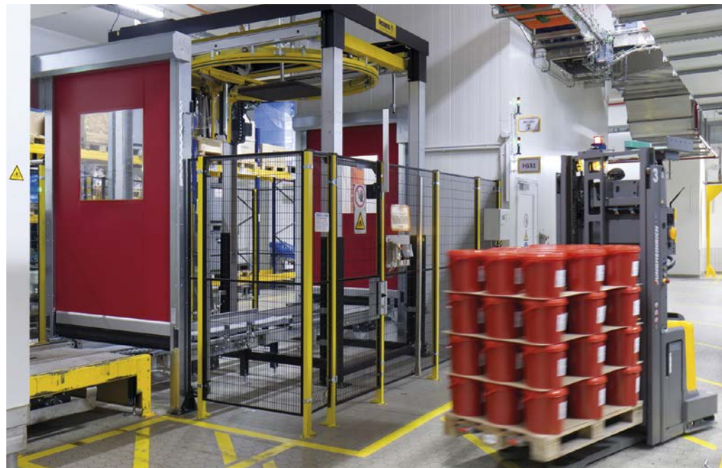
EFA-SRT high-speed roll-up doors separate different production areas from each other (photo: EFAFLEX)
