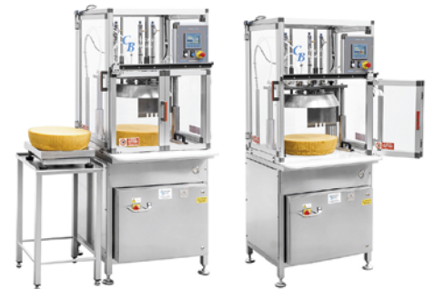
ROCK 20 PLUS AUTOMATIC PORTIONING MACHINE TO CUT THE CHEESE WITH VARIABLE AND FIXED WEIGHT WORK PROGRAMS.
